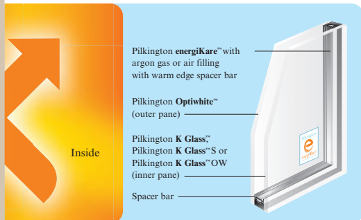
Cross section Pilkington energiKare™ unit
