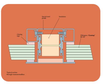
Pilkington **Pyrostop**<sup>™</sup> in Multi-pane Steel Screen. 60 minutes integrity and 60 minutes insulation. Fire Test Reference: WARRES 113978.
