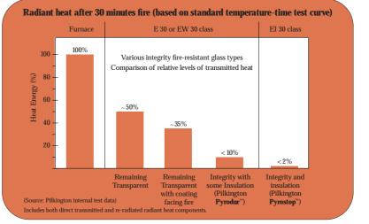
Controlling radiant heat is a significant factor in saving lives as well as an important mechanism influencing the spread of fire. Although radiant heat reduction is not a requirement in UK regulations, comparison of transmitted radiant heat levels does provide a ready means of comparing different integrity glazings.
