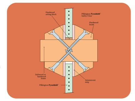
Pilkington **Pyroshield**<sup>∞</sup> Safety Clear in Softwood Timber Screen. 30 minutes integrity. Fire Test Reference: WARRES 70068.
